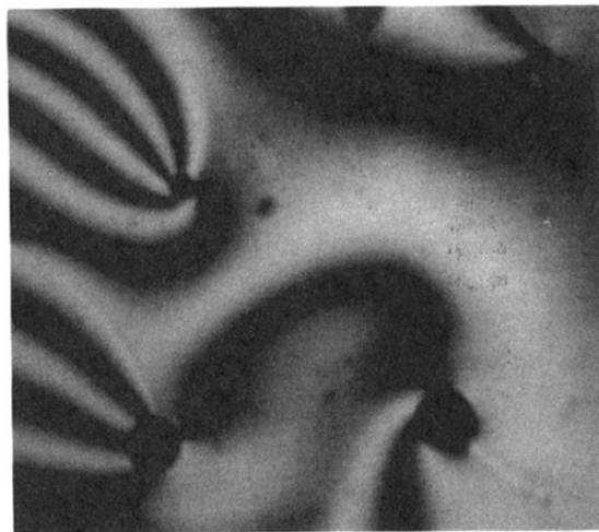
FIG. 15. Experimental view of the isotropic nucleation at the cores of defects in a semithin film of para azoxyanisole, at a temperature slightly above T_c = 136^\circ\text{C} .
