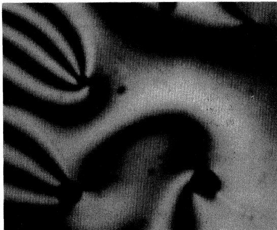
FIG. 15. Experimental view of the isotropic nucleation at the cores of defects in a semithin film of para azoxyanisole, at a temperature slightly above T_c = 136^\circ\text{C} .
